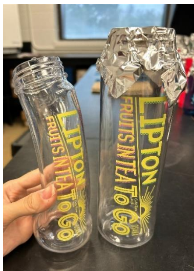
Figure 3: Example of PET bottle after 20 cycles of dishwasher (left) compared to the same type of bottle initially (right).
